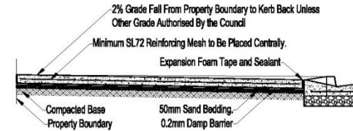
Vehicle Crossover Section View
